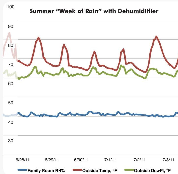
After installation of an Ultra-Aire 90H Whole House Ventilating Dehumidifier, RH stabilized in the 50% range.
